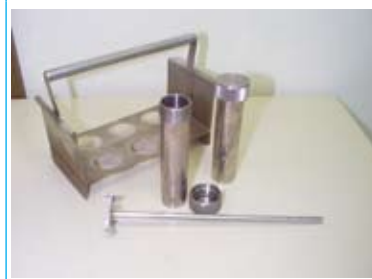
Figure 3 Equipment used in the CSIRO heat stability test. (Kieseker & Aitken 1988)
