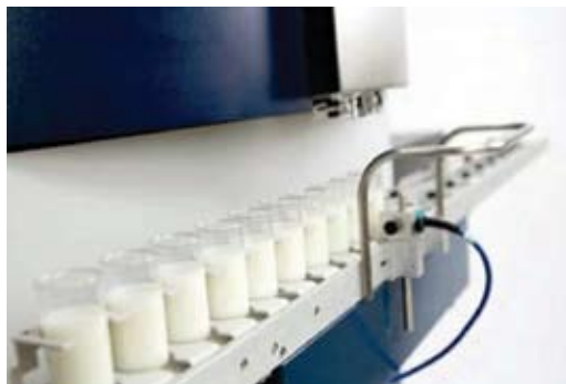
Close-up of the sample conveyor and automatic sampling device used on automated Foss milk testing equipment
