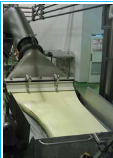
Pizza cheese during the stretching process of manufacture
