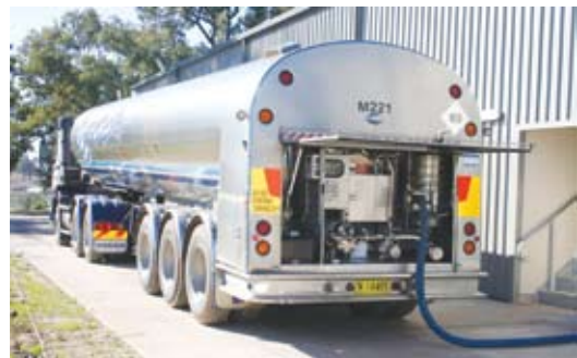
Milk being pumped from a farm storage tank into a collection tanker
