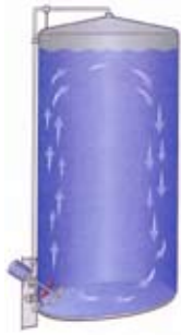
Silo for storage of raw milk at a processing factory, with mechanical agitation of the milk
