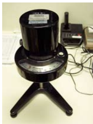
Brookfield viscometer used for accurate viscosity testing.
