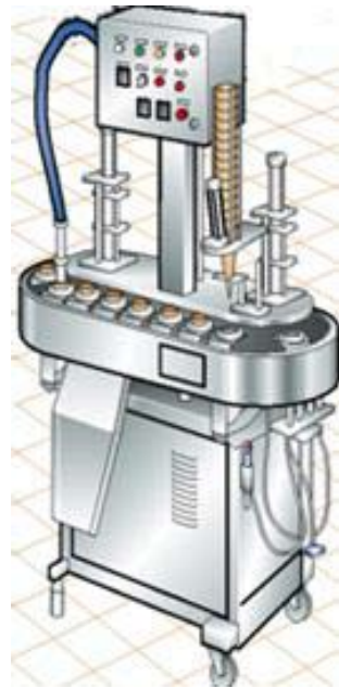
Cup and cone packaging machine (Dairy processing
