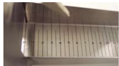
Bostwick consistometer used for rapid estimates of viscosity
