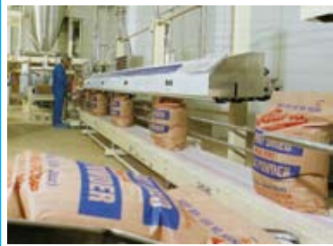
Figure 11 Shows the sealing section of a 25kg bagging line
