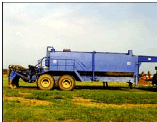
Sludge Injection Tanker
