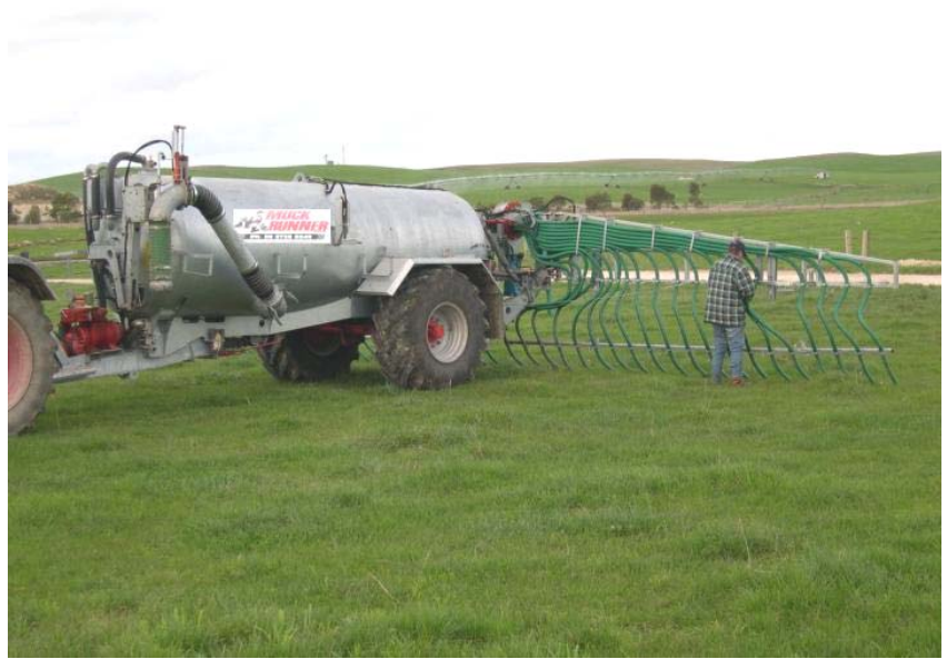
An example of a slurry tanker fitted with a dribble bar effluent spreading system
