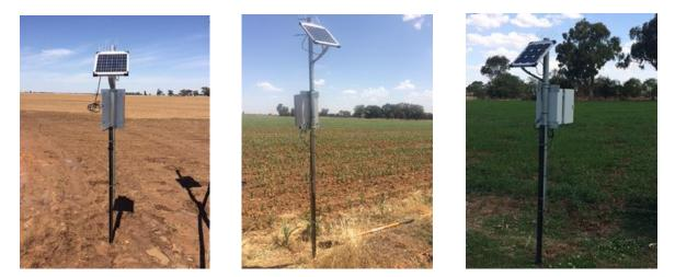
C capacitance - soil moisture probes installed in the Riverina region.
