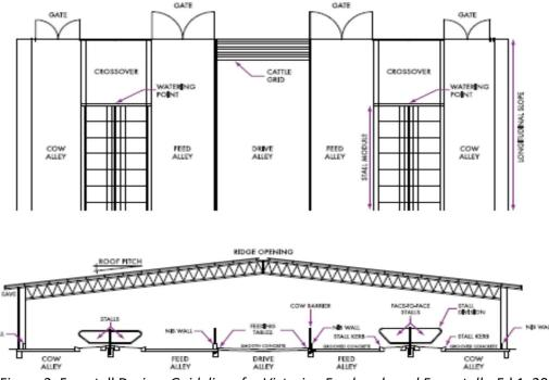
Figure 2. Freestall Design. Guidelines for Victorian Feed-pads and Free-stalls. Ed 1. 2010. Vic DPI (21)
