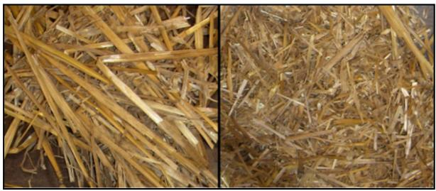
Figure 18. Chopped straw (left) and straw run through hammer mill with 3/4" screen (right). Source Bewley et al (Ref. 17)
