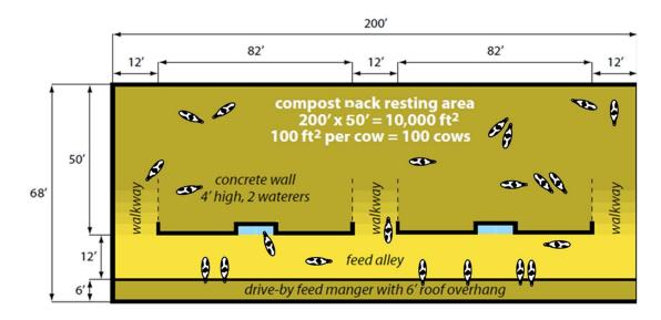
Figure 12; Minnesota type composting barn layout in USA, with concrete alleyway, watering troughs and fed bunk separate from the compost bed. Source; Endres et al. (15)
