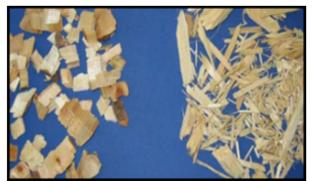
Figure 17. Wood chips produced with sharp (left) and blunt hammer (right) (Source Ref. 17)
