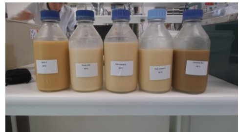
Skim milk, goat's milk, full cream cow's milk (X2) and lactose-reduced milk, after storage at 50 °C for 4 months
