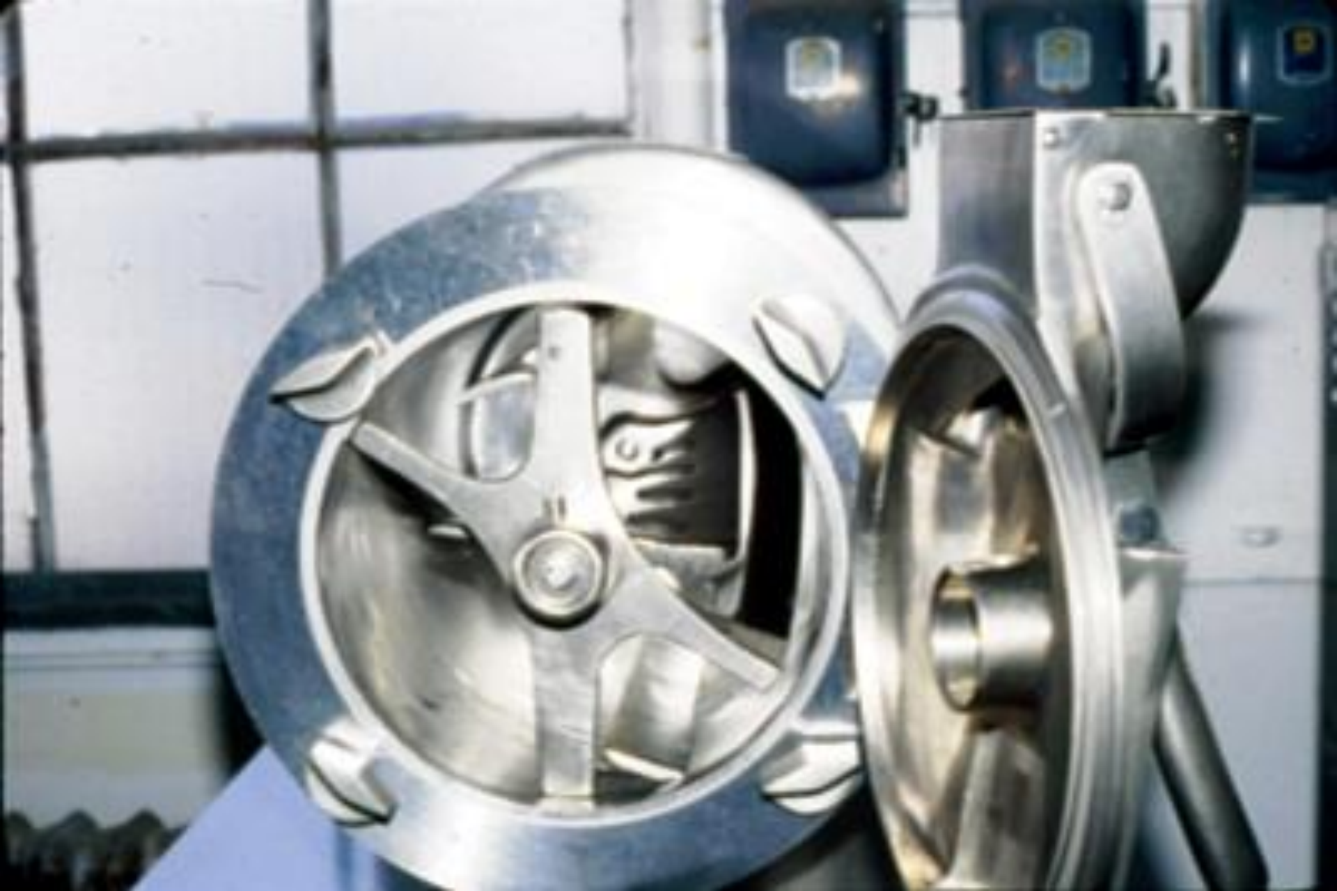
Dasher and scraper blades in a batch ice cream freezer
