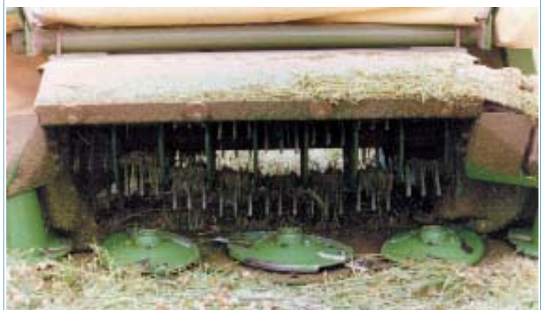
Disc mower, with flail conditioner.
