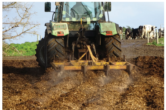
Chisel plough used to till a large compost bedding pack
