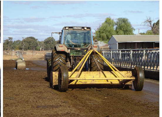
Drylot feed alley being dry scraped
