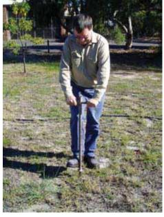
Figure 3.2 A sampling pogo is a metal tube about 2.5 cm in diameter that is pushed into the soil to a depth of 10 cm.
