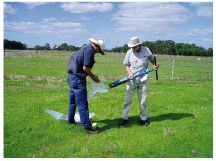
Figure 3.1 Soil sampling using an auger
