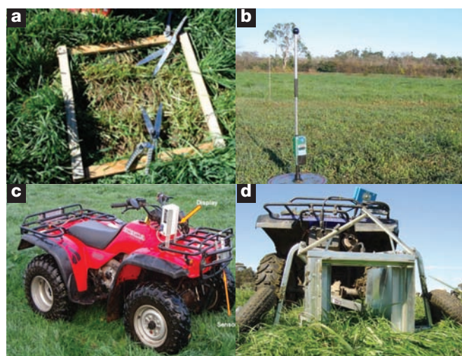
Figure 2. Methods to estimate pasture cover (a) cut pasture, (b) rising plate meter, (c) Ellinbank automatic pasture reader, and (d) rapid pasture meter (C-Dax).
